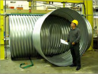
2.40m Ø "T" section under load test at BBA
